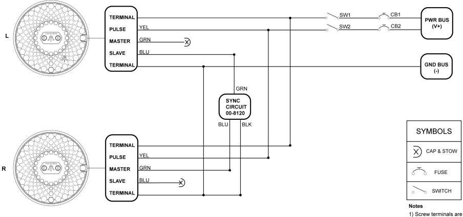
1) Screw terminals are not polarity sensitive
